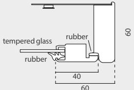
Aluminium thickness 1.5mm to 1.8mm
