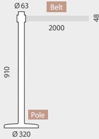
STAINLESS STEEL BARRIER POLE WITH RETRACTABLE BELT
