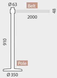
STACKABLE BARRIER POLE WITH RETRACTABLE BELT
