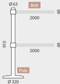
BARRIER POLE DOUBLE RETRACTABLE BELT
